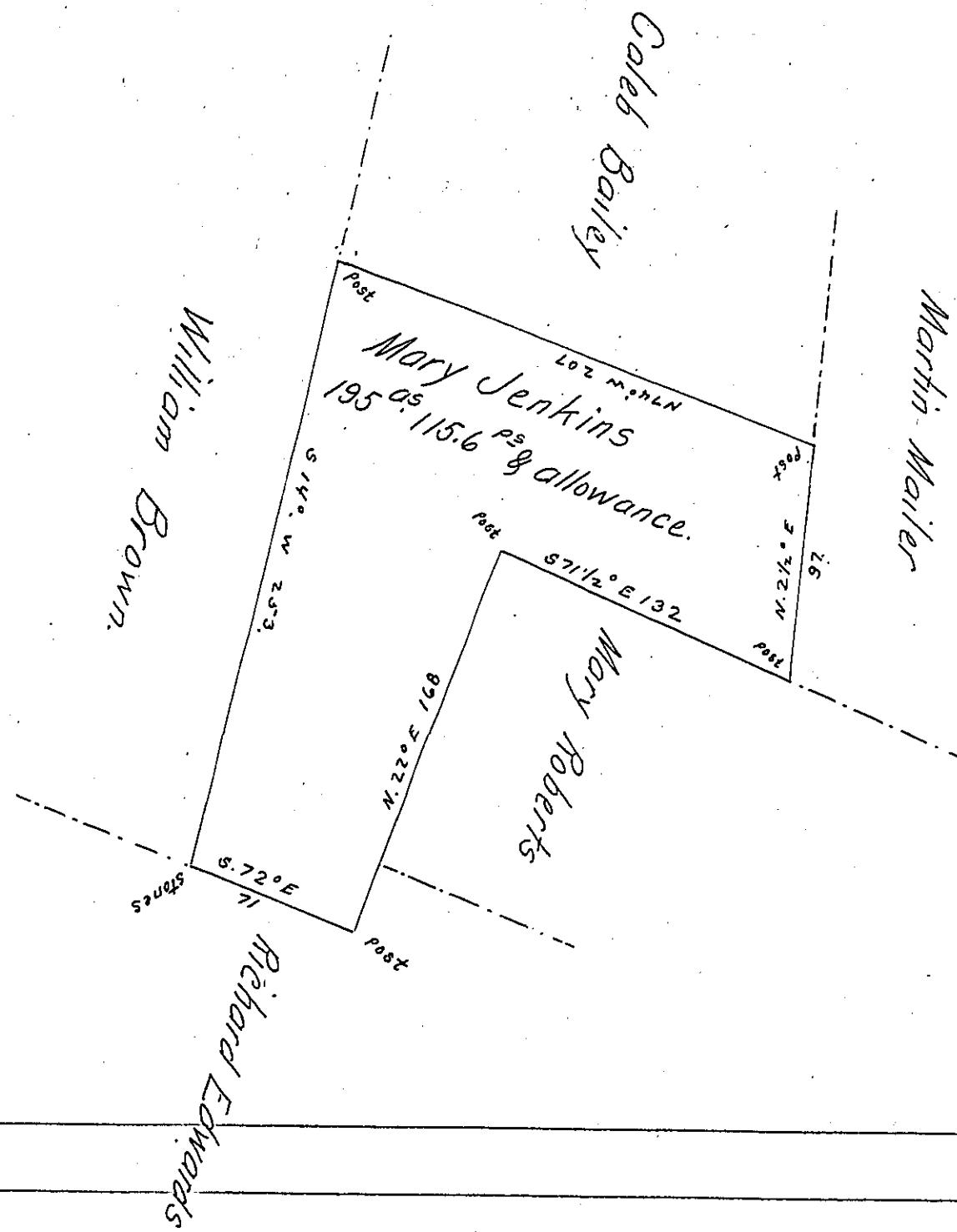
Draft of a tract of land Containing 195 Acres 115.6 perches and allowance of Six per Cent for Roads &c Situate in Burnside Township Clearfield County Surveyed for Simon and Alexander Fulton At the instance of Aaron W. Patchin Dec. 31<sup>st</sup> 1874 being the residue of a tract Originally Surveyed on a Warrant Dated 3<sup>d</sup> of Aug. 1773 and granted to Mary Jenkins
